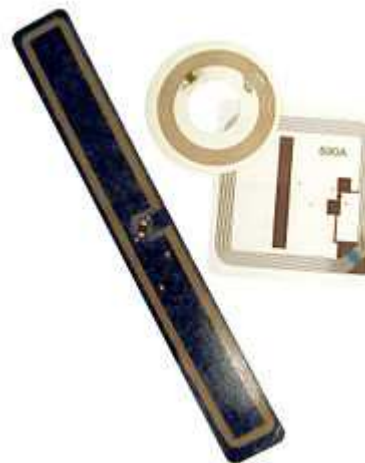
RFID tags used in libraries: square book tag, round CD/DVD tag and rectangular VHS tag.[1]
